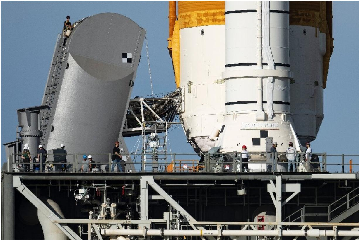
Engineers work on the Tail Service Mast Umbilical of the Artemis I unmanned lunar rocket as it sits on launch pad 39B at NASA's Kennedy Space Center.
