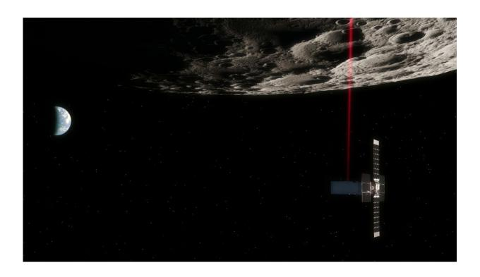
This illustration shows NASA's Lunar Flashlight using its four-laser reflectometer to search for surface water ice as it makes a close approach over the Moon's South Pole. Credit: NASA/JPL-Caltech
