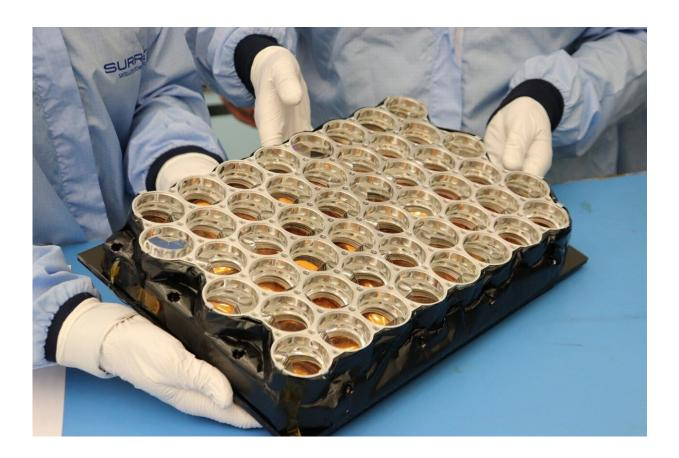
Laser Retroreflector Array. Credit: SSTL
