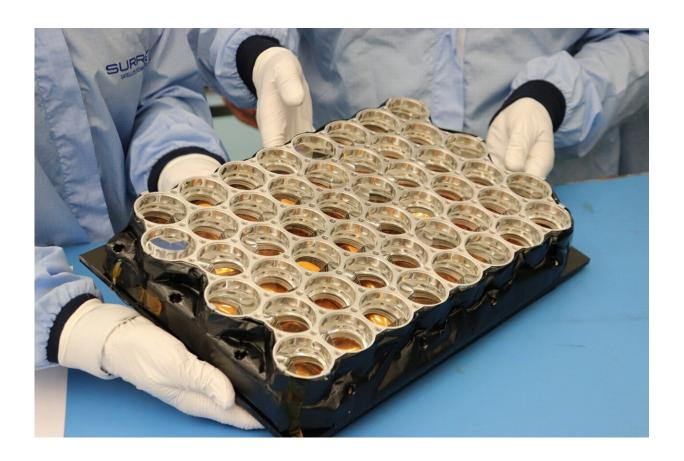
Laser Retroreflector Array. Credit: SSTL
