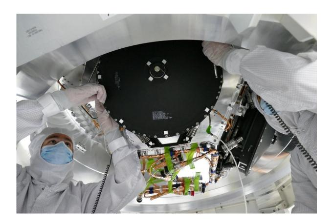
Engineers install 2-foot-wide reaction wheels onto the main body of NASA's Europa Clipper spacecraft. The orbiter is in its assembly, test, and launch operations phase in preparation for a 2024 launch. Credit: NASA/JPL-Caltech
