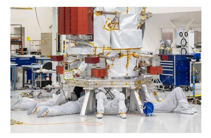
Engineers and technicians work together to install reaction wheels on the underside of the main body of NASA's Europa Clipper spacecraft, which is in its assembly, test, and launch operations phase. Credit: NASA/JPL-Caltech
