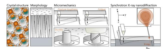
Assessing the fracture and fatigue resistance of nanostructured thin films
