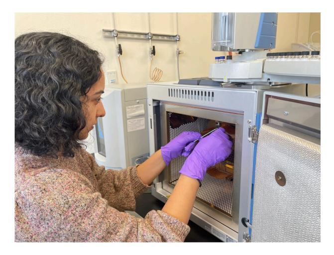
Bhattacharya performs maintenance on her gas chromatograph, a key piece of lab equipment that allows her to quantify the concentrations of leaf waxes in ancient sediments. Credit: Syracuse University
