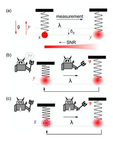
Schematic information engine. (a) Noisy detector measures position y of the bead, actually located at x. Ratchet based on either (b) noisy position measurement y or (c) Bayesian position estimate  $_X$  (blue dashed circle). Credit: *Physical Review Letters* (2022). DOI: 10.1103/PhysRevLett.129.130601
