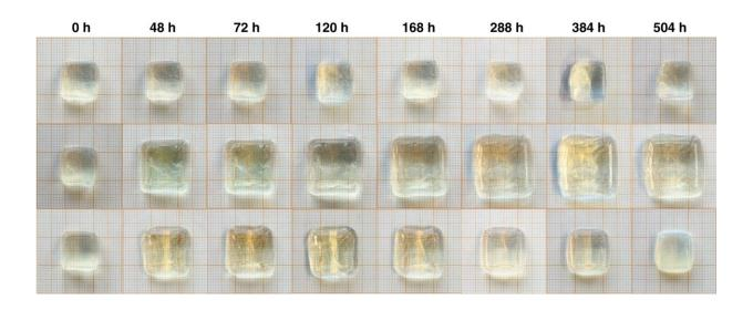
Time-lapse photo series of a hydrogel with fuel added (middle row) compared with a control hydrogel to which nothing has been added (top row), over a three-week period (504 hours). The bottom row shows a hydrogel that changes shape independently when two different types of fuel are added. Credit: TU Delft
