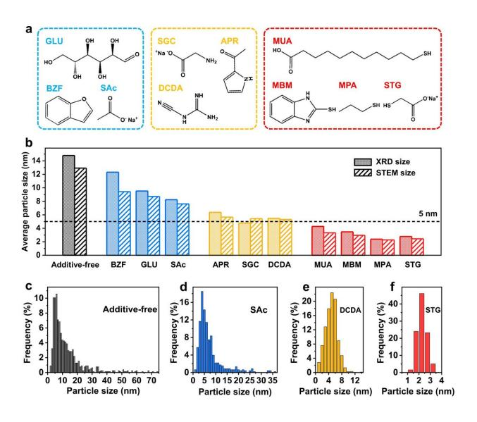
Screening small molecules for suppressing metal sintering. (a) The structures of the molecules used as additives for suppressing metal sintering. (b) XRD (solid shadow column) and STEM (twill stripes column) sizes of PtCo particles with
