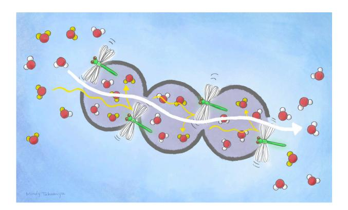
Incorporating dragonfly-shaped gate molecules into PCP/MOFs makes it a hundred times more efficient than before to separate water from heavy water. The two have been difficult to separate due to their similar properties. Credit: Mindy Takamiya/Kyoto University iCeMS
