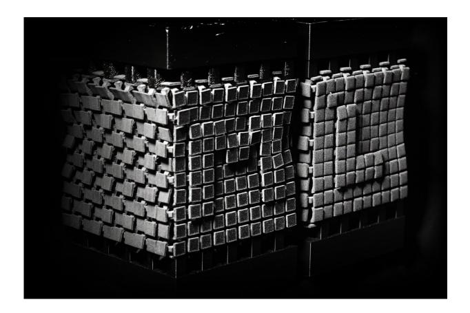
Two combinatorial mechanical metamaterials designed in such a way that the letters M and L bulge out in the front when being squeezed between two plates (top and bottom). Designing novel metamaterials such as this is made easy by AI. Credit: Daan Haver and Yao Du, University of Amsterdam
