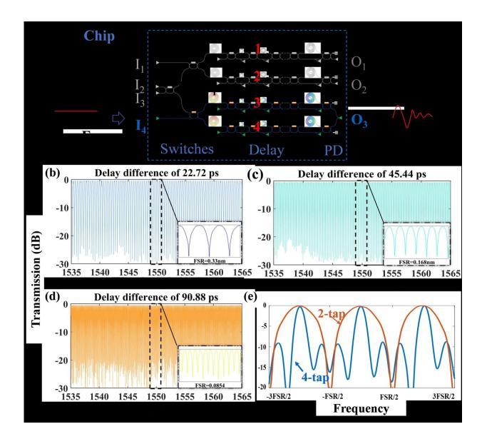
Principle of arbitrary filtering operation (Input from port I4, and output from port O3). Measurements of filter spectral responses: (b)-(d) demonstrations of the FSR tunability for the filter; (e) demonstrations of passband shaping for the filter. Credit: Compuscript Ltd
