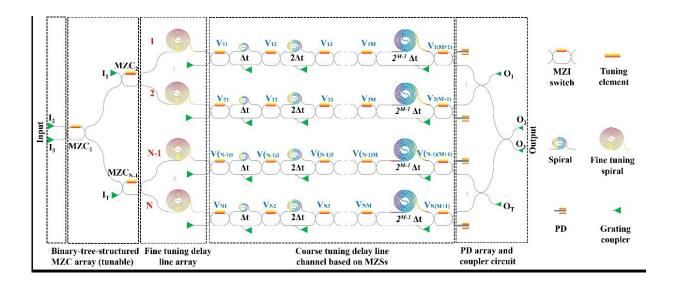
Schematic of an on-chip optical signal processor. Credit: Compuscript Ltd
