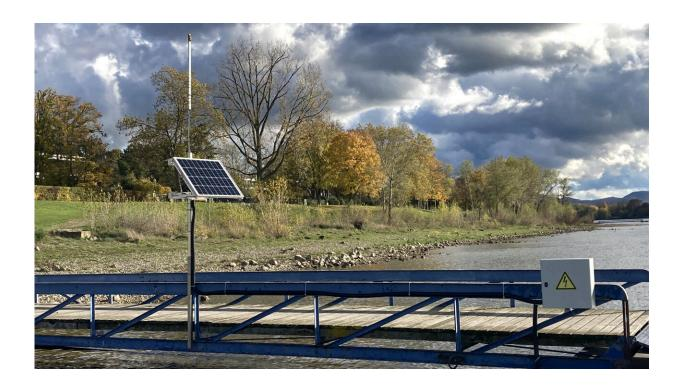
The water level sensor can be operated with solar cells and then works completely stand alone with no maintenance. Credit: Makan Karegar/University of Bonn
