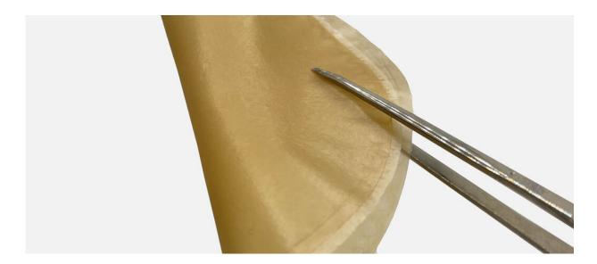
The strength of the composite material was higher than that of nanocellulose paper alone or polymer alone in both dry and wet conditions. Credit: Aalto University / Erfan Kimiaei
