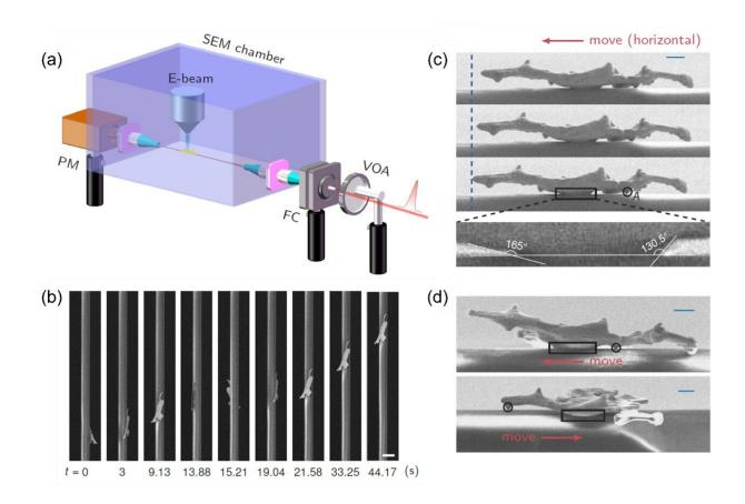
Experimental observations of an Sb<sub>2</sub>Te<sub>3</sub> plate moving spirally around a microfiber. (a) Sketch of experimental setup implemented in a vacuum chamber. VOA, variable optical attenuator; FC, fiber coupler; MF, microfiber; and PM, power meter. (b) Temporal sequencing SEM images of an Sb<sub>2</sub>Te<sub>3</sub> plate moving around a microfiber when the average power of the driving laser is below the threshold power. In this case, the asymmetric reflection of the opto-thermo-
