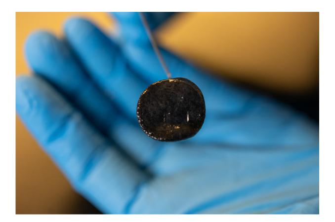
Pucklike bioelectronics designed at Rice University contain programmable bacteria and are attached to an electrode that delivers a signal when they detect a target contaminant, enabling real-time sensing. Credit: Brandon Martin/Rice University
