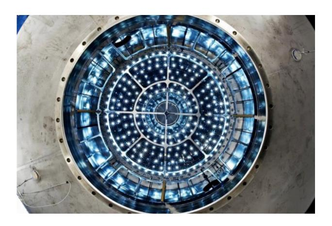
The Cosmics Leaving Outdoor Droplets (CLOUD) experiment at CERN, Geneva uses an ultraclean chamber facility to study how gases form new particles (nucleation), and grow to affect cloud formation. The primary goal of CLOUD is to understand the influence of galactic cosmic rays (GCRs) on aerosols and clouds, and their implications for climate. Credit: CERN
