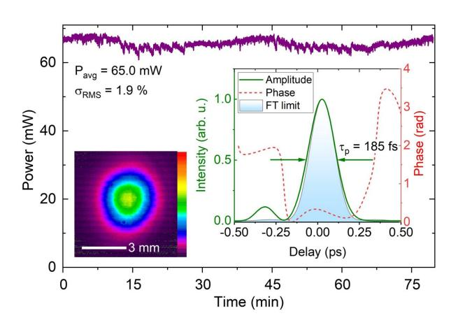
Characterization of the OPCPA pulse performance at 11.4 µm. Long-term pulse stability measurement. The average power is 65 mW, the standard deviation 6\_RMS=1.9%. Left inset: Far-field intensity distribution. Right inset: Retrieved temporal pulse shape of the few-cycle pulse. Credit: *Optica* (2022). DOI: 10.1364/OPTICA.472650
