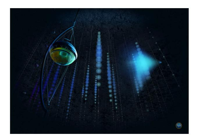
When a neutrino interacts with molecules in the clear Antarctic ice, it produces secondary particles that leave a trace of blue light as they travel through the IceCube detector. Credit: Nicolle R. Fuller, IceCube/NSF
