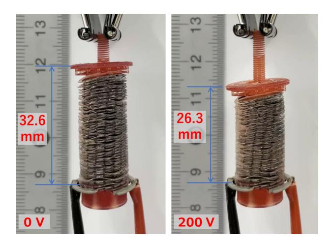
Figure 2. The use of the ferroelectric medium generated forces sufficient to achieve a contraction of 6.3 mm with the application of 200 V. The device was also observed to move slightly at 18 V, indicating that it can be powered by a battery. Credit: *Advanced Physics Research*
