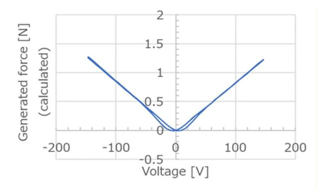
Figure 1. Since the generated force in ferroelectric media is directly proportional to the applied voltage, they can be used to generate much higher forces at lower voltages, making their use in electrostatic actuators a feasible option. Credit: *Advanced Physics Research*
