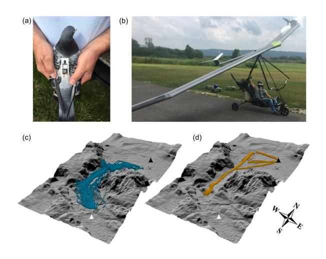
The logging platforms used in this study and corresponding flight tracks. (a) The combined logger unit used on the pigeon's back, (b) the ultralight, (c) pigeon tracks and (d) ultralight flight legs. Black and white triangles indicate the location of the release site and the loft, respectively. The parts of the tracks where pigeons performed orientation circles near the release site or loft, and the
