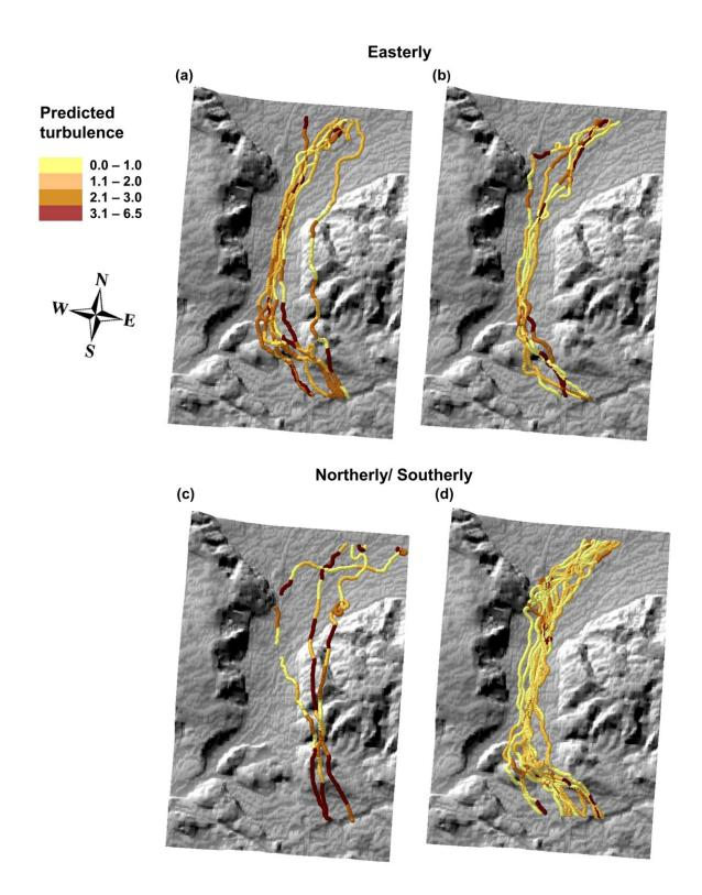
Spatial variation in turbulence as predicted from the fluctuations in pressure recorded onboard. Predictions were made for a) highly turbulent conditions and
