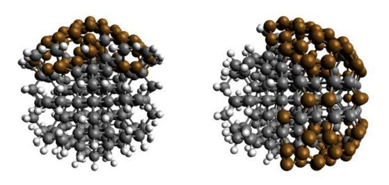
The illustration shows two variants of nanodiamond materials with different surfaces:  $C_{230}H_{106}$  on the left,  $C_{286}H_{68}$  on the right. Sp3 C atoms (diamond) black, sp3x C atoms (fullerene-like) brown, H atoms: Light grey. When the surface is partially covered by hydrogen atoms, nanodiamonds can absorb light in the visible range and emit electrons into solution. Credit: T. Kirschbaum / HZB
