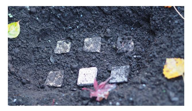
The biofoam starts breaking down in the soil within a few weeks. Photo shows four biofoam samples (top row and bottom left) and two petrochemical foam samples (bottom right and center) after a month in the ground. Credit: Lou Bosshart/UBC
