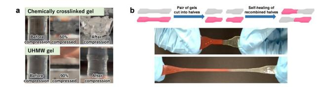
(a) Comparison of compressibility between a chemically crosslinked gel and a UHMW gel. (b) Schematic showing UHMW gels' ability to be recombined and the photos of recombined gels being stretched. Credit: Ryota Tamate / National Institute for Materials Science
