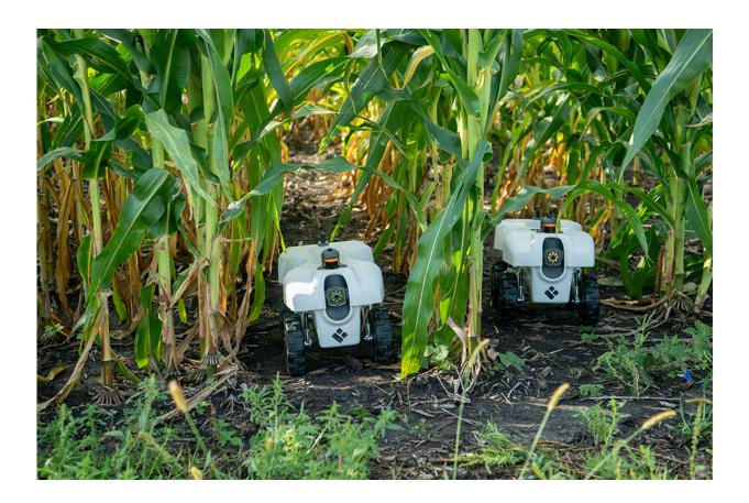
Small robots can move under the canopy to perform tasks such as fertilization, seeding, diagnostics, and mechanical weeding. Credit: University of Illinois
