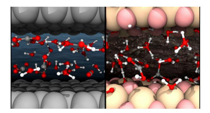
Left: the solution is confined by graphene. Right: the solution is confined by stishovite  $(SiO_2)$ . The white, gray, red, and pink balls are the hydrogen, carbon, oxygen, and silicon atoms, respectively. Credit: HKUST
