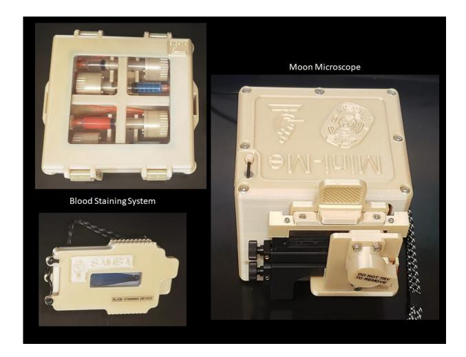
Staining reagents and syringe storage box (upper left), staining device (lower left), and miniature microscope (right) for the Moon Microscope investigation. Credit: NASA JSC Immunology/Virology Laboratory
