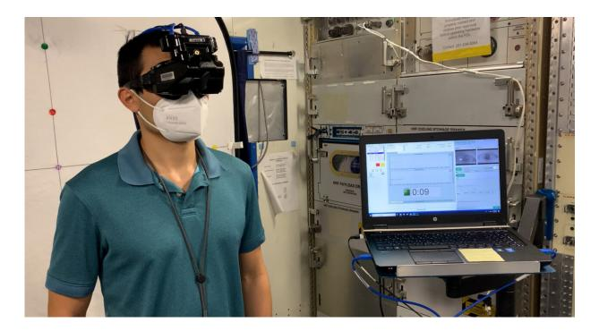
Ground testing of the Falcon Goggles. This technology captures high-speed video of a subject's eyes, providing precise data on ocular alignment and balance and could guide researchers in developing ways to help crew members adapt to different gravity conditions on future exploration missions. Credit: NASA
