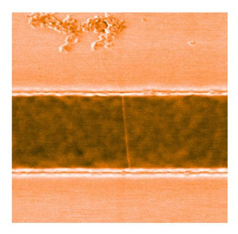
A carbon nanotube suspended across a trench in a silicon substrate. By developing a method that allows such suspended nanotubes to be functionalized with organic molecules, RIKEN researchers have enhanced their usefulness for sources of single photons. Credit: Reproduced from Ref. 1 and licensed under <u>CC BY 4.0</u> © 2022 D. Kozawa et al.
