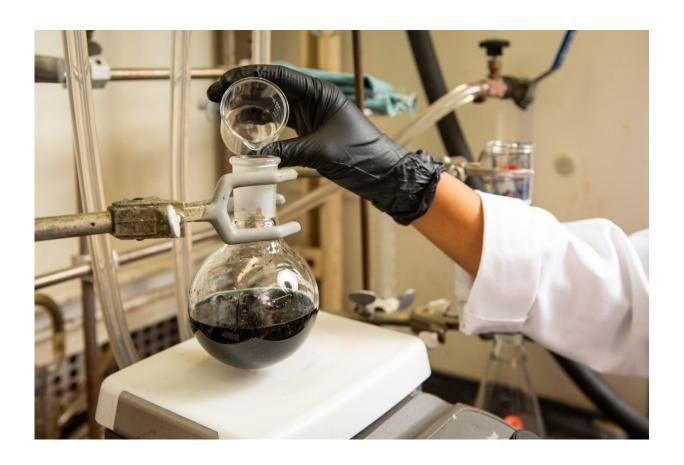
Ananya Saju, UB PhD student in chemistry, carries out the reaction that is used to stabilize manganese trichloride. The work involves fixing a stabilizing agent to MnCl<sub>3</sub> that prevents it from indiscriminately shedding chlorine atoms, as it
