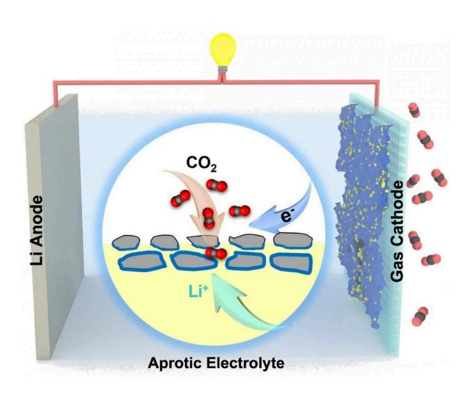
Figure 1. Schematic illustration of the aprotic Li-CO2 battery. Credit: *Proceedings of the National Academy of Sciences* (2022). DOI: 10.1073/pnas.2204666119
