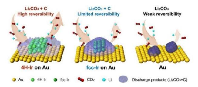
Figure 2. Three different kinds of electrochemical reaction kinetics on Au@4H-Ir, Au@fcc-Ir and pure Au (right panel) in an aprotic Li-CO<sub>2</sub> battery. Credit: *Proceedings of the National Academy of Sciences* (2022). DOI: 10.1073/pnas.2204666119
