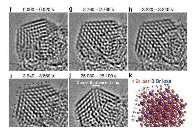
Stills from the video captured using "cinematic chemistry" of the blue quantum dot, including an illustration showing the atomic arrangement of the sample. Credit: ©2022 Nakamura et al.
