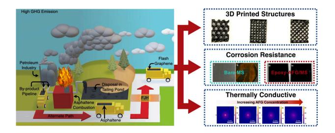
Researchers at Rice University are pursuing the "sustainable valorization" of asphaltene by turning it into graphene useful for composite materials. Credit: M.A.S.R. Saadi/Rice University
