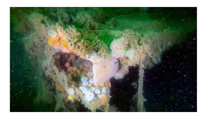
Torn deck plating of the V 1302 John Mahn that was damaged by the bomb that hit amidships. Credit: VLIZ
