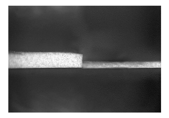
Purdue University researchers have created a new formula for the world's whitest paint, making it thinner and lighter. The previous iteration (left) required a layer 0.4 millimeters thick to achieve sub-ambient radiant cooling. The new formulation can achieve similar cooling with a layer just 0.15 millimeters thick. This is thin and light enough for its radiant cooling effects to be applied to vehicles like cars, trains and airplanes. Credit: Purdue University, Andrea Felicelli
