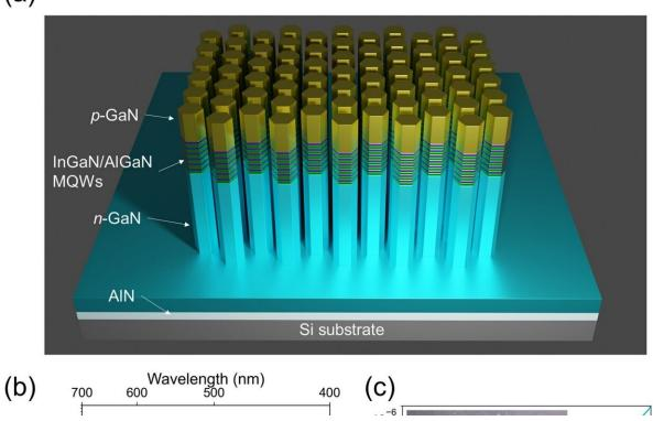
(a) Schematic of the InGaN/AGaN multiple-quantum-well nanowire array. (b) The peak wavelength of the device's electroluminescence stays constant over one order of magnitude of change in current injection. (c) The current voltage characteristics of a device that shows good rectification ratio and strong green emission visible to the eyes. Credit: *Light: Science & Applications* (2022). DOI: 10.1038/s41377-022-00985-4
