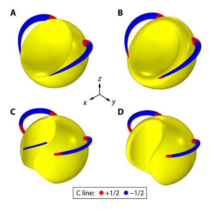
Effect of singular edges. (A and B) The C lines generated by a sphere with sharp circular edge and with the sharp edge smoothed out, respectively. (C and D) The C lines generated by a sphere with sharp irregular edge (created by removing a cylindrical portion from the sphere) and with the sharp edge smoothed out, respectively. There are two C lines in (A), (B), and (D) and four C lines in (C). Credit: *Science Advances* (2022). DOI: 10.1126/sciadv.abq0910
