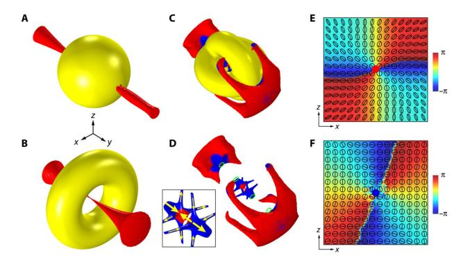
Higher-order C lines due to generalized rotational symmetry. (A and B) Higher-order C lines with index Ipl = +1 generated by a sphere and a torus, respectively. (C and D) Higher-order C lines generated by a torus nexus with C4 rotational symmetry. The torus nexus is removed in (D) to enable a clear view of the internal structures of the C lines. The green circles mark the four C points with
