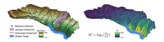
Conceptual diagram of Index of Connectivity calculation, which utilizes weighted upstream and downstream components. Credit: Admin Husic
