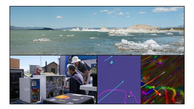
Counterclockwise from top: California's Mono Lake was the site of a field test for JPL's Ocean Worlds Life Surveyor. A suite of eight instruments designed to detect life in liquid samples from icy moons, OWLS can autonomously track lifelike movement in water flowing past its microscopes. Credit: NASA/JPL-Caltech
