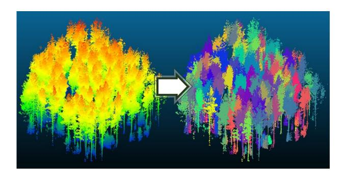
This image shows the input and output data of the tree segmentation algorithm. The input data (left) is colored by elevation. The results of the algorithm (right) use color to segment each tree from the point cloud. Credit: Purdue University photo/Joshua Carpenter
