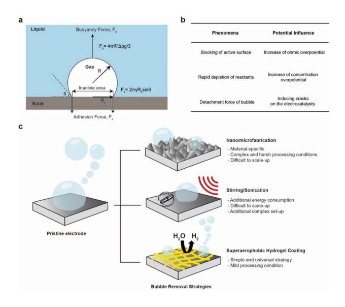
The scheme for a mechanism of bubble-detachment. a) Normal flat electrode, b)
