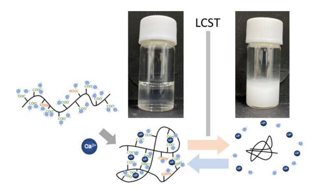
The novel thermoresponsive polymer was created by adding ions to polymers and aqueous solutions. Its thermoresponsiveness can easily be controlled by changing the type and mixing ratio of ionic species. Credit: Harada, OMU
