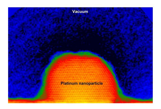
Ultrahigh sensitivity and precision electron holography measurements around a platinum nanoparticle like the one shown here have allowed scientists to count the net charge in a single catalyst nanoparticle with a precision of just one electron for the first time. Credit: Murakami Lab, Kyushu University
