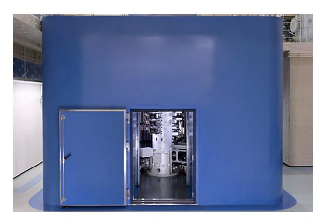
Since 1966, Hitachi has been developing the holography electron microscope as an instrument for the direct observation of electric and magnetic fields in extremely small regions, and in 2014, developed a 1.2-MV atomic-resolution holography electron microscope with a grant under the Funding Program for World-Leading Innovative R&D on Science and Technology (the "FIRST Program"), a national project sponsored by the Japanese government. Credit: Hitachi, Ltd.
