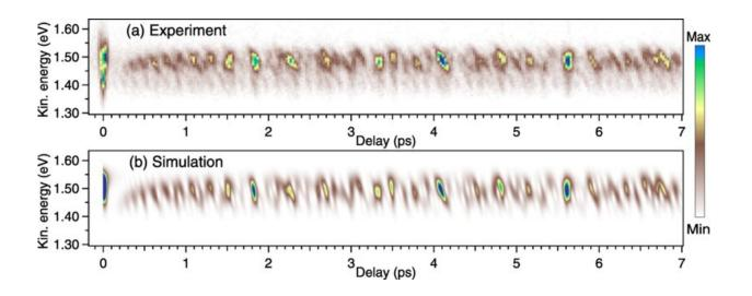
(a) Experimental photoelectron yield map as a function of the delay between XUV and NIR pulses. (b) Simulated photoelectron yield map using 24.587 eV XUV central energy and 0.09433 eV XUV bandwidth. Credit: *Physical Review Research* (2022). DOI: 10.1103/PhysRevResearch.4.043041
