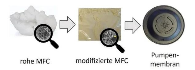
It is a challenge to blend microfibrillated cellulose (MFC) with hydrophobic, i.e. water-repellent, rubbers. Credit: Empa / Daetwyler Schweiz AG
