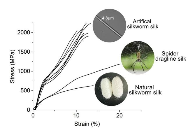
Stress-strain curves of representative artificial and natural silks. Credit: Jingxia Wang, Tiantian Fan, & Zhi Lin
