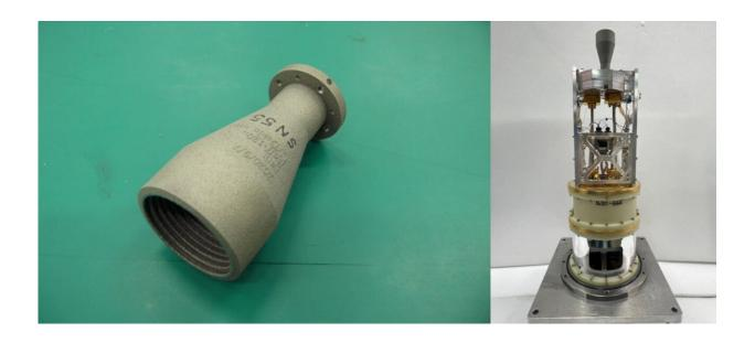
A 3D-printed corrugated horn (left). A Band 1 receiver with the all-metal 3D-printed corrugated horn installed (right). Credit: NAOJ, ASIAA
