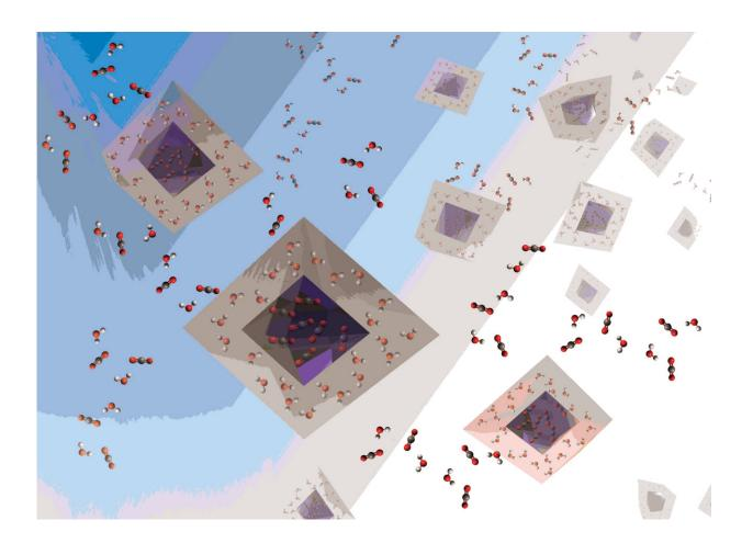
The MOF would have a core-shell design, meaning carbon dioxide would be trapped in the core, while the shell is able to block other gasses, specifically water. The shell and the core would be made from different MOF materials, with the shell MOF designed to slow down water and the core MOF designed to bind  $CO_2$ . Credit: The University of Pittsburgh
