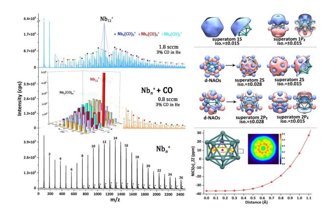
(Left) Typical mass spectra of the cationic niobium clusters produced by a homemade magnetron sputtering (MagS) source and collected by a customized triple quadrupole mass spectrometer (TQMS), and after reacting with different dose of reactants (3% CO in He). The inset shows the intensity of  $Nb_n(CO)_m^+$  (n=7-16, m=0-8) after  $Nb_n^+$  clusters react with the CO reactant. (Right) A composition of the superatomic 1S and 1Pz orbitals, with 2S and 2Pz orbitals in
