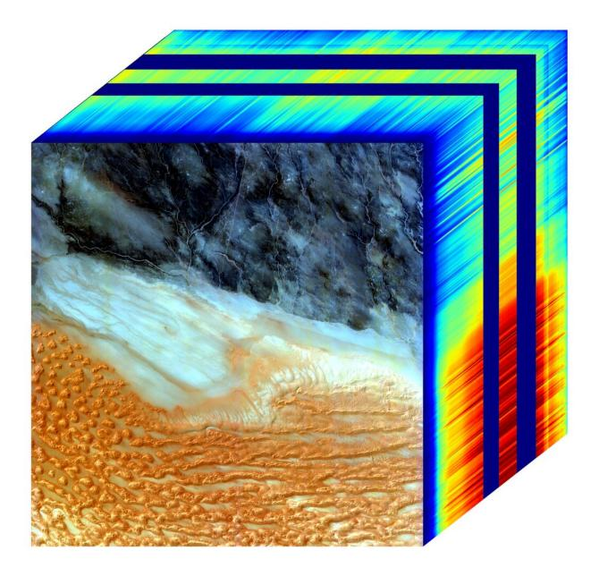
The image cube's front panel is a true-color view of part of southwestern Libya observed by NASA's EMIT mission. The side panels depict the spectral fingerprints for every point in the image, showing kaolinite, a reflective clay mineral, and goethite and hematite, iron oxides that absorb heat. Credit: NASA/JPL-Caltech
