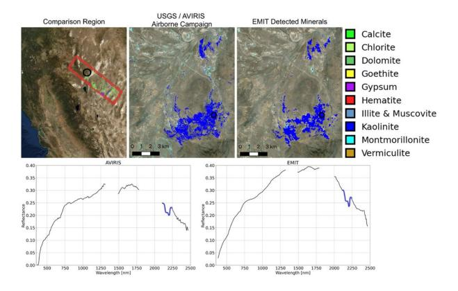
NASA's EMIT mission recently gathered mineral spectra in northwest Nevada that match what the agency's AVIRIS instrument found in 2018, helping to confirm EMIT's accuracy. Both instruments found areas dominated by kaolinite, a reflective clay mineral whose particles can cool the air when airborne. Credit: NASA/JPL-Caltech/USGS
