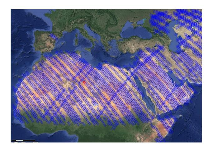
Installed on the space station in July 2022, EMIT orbits Earth about once every 90 minutes, to map the world's mineral-dust sources. This includes the Sahara, where it recently gathered data on three minerals—goethite, hematite, and kaolinite—in an area of southwest Libya marked by the red box. Credit: NASA/JPL-Caltech
