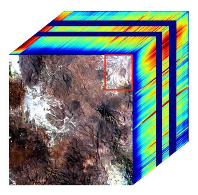
This image cube shows the true-color view of an area in northwest Nevada observed by NASA's EMIT imaging spectrometer. The side panels depict the spectral fingerprint for each point in the image. The cube shows the presence of kaolinite, a light-colored clay mineral that reflects sunlight. Credit: NASA/JPL-Caltech/USGS
