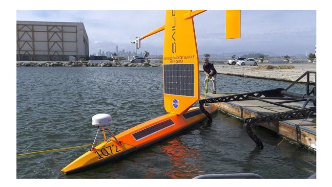
Saildrones like the one seen here are part of the fleet of autonomous marine research vessels measuring factors such as ocean currents, salinity, and chlorophyll content as part of NASA's S-MODE field campaign. Credit: NASA
